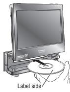
**Caution:** When the disc is inserted or ejected, to prevent disc scratches never exert any downward force on the disc.
